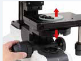
Adjust for tall sample by up/down motion of stage
